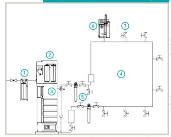
**A total water purification** system requires the main water purification system to be integrated into a centralized system. For example:
